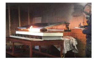
The tests were carried out according to the CLC /TR 50670<sup>16</sup> principles. A gas burner was placed and ignited between the PV panel and the roof covering.
