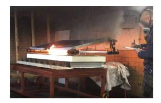
The tests were carried out according to the CLC /TR 50670<sup>15</sup> principles. A gas burner was
